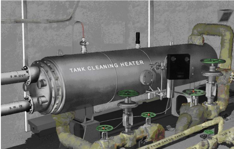
Tank Cleaning Heater
