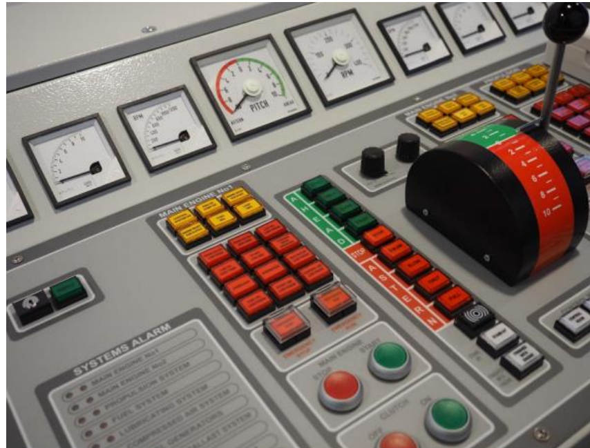
The UNITEST single console is an engine room simulator with a single desktop hardware console.
