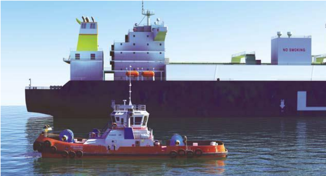
Use of Tug to assist vessel berthing
